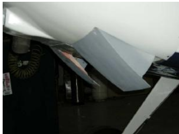
Figure 7. Cessna 182 Cowling Flaps
