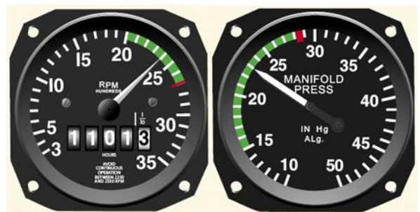
Figure 6. RPM and Manifold Pressure Gage.
